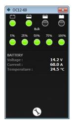
This panel shows the charge progress bar, the output current indication bar and the present battery voltage, current and temperature. When the temperature sensor is not connected, the temperature reading shows --.-°C.
