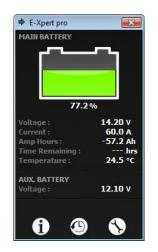
As you can see in the above picture, this panel shows the present battery voltage, current, temperature and state-of-charge as well as the amount of Amp Hours removed from the battery and the time remaining until the battery needs to be recharged.
