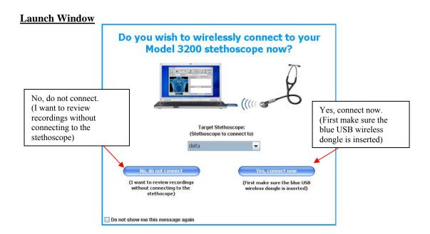
To connect to a Model 3200 stethoscope for the first time, you must follow the steps below to "pair" the stethoscope with StethAssist.
