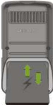
When installing the battery, insert the metal teeth at the top of the battery into corresponding slot of the mobile phone. Press the battery firmly in place. Install the battery with the phone switched off.
