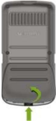
Lift the bottom of the battery and slide the battery out.
