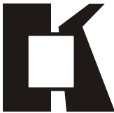
"K" Base fits to the bottom of the VP-701SC for Vertical Desktop Mounting
