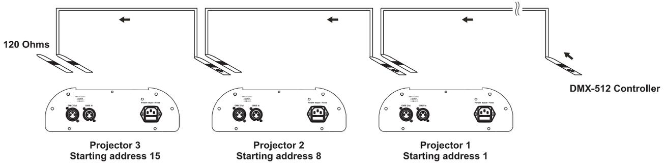
**! The wires must not come into contact with each other, otherwise the fixtures will not work at all, or will not work properly. !**
