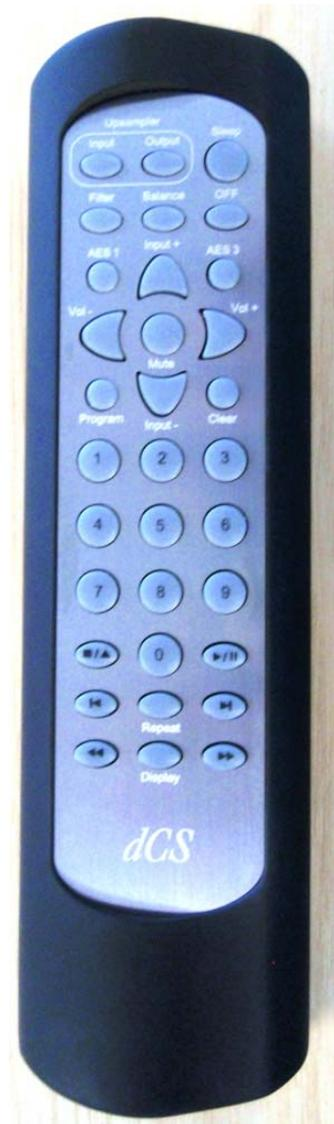
Hold down the **Sleep** button for 2 seconds to set the system to sleep mode. Press the **Sleep** button again to return to normal operation.
