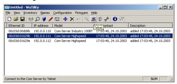
This utility makes it convenient to locate the Synchronous Com-Servers in the network. It can be downloaded from the website of the module manufacturer; <a href="www.WuT.de">www.WuT.de</a>
