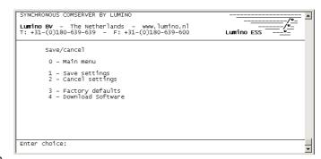
**Download software**: Select this option only when the firmware upgrade utility with a new firmware version is available and started. The firmware upgrade utility should come with documentation on the upgrade procedure.
