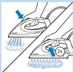
There are two steam boost functions for removing stubborn creases.
