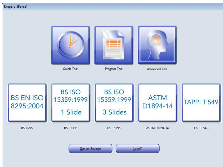
All supplied programs are listed under 'Advanced Test' in the Test Library, and any can be assigned to, or removed from, a Favourites position. (See the Emperor™ software manuals for full details.)
