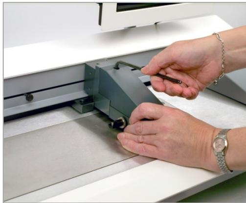
Attaching and removing the loadcell
