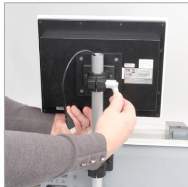
Push the button on the grey handle to lift and turn it as required, and to leave it tidily.
