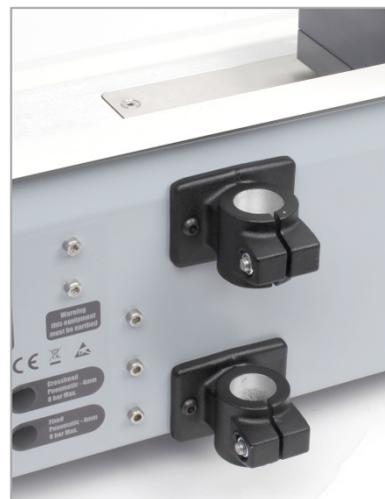
Insert the pillar into the brackets and tighten the brackets very firmly onto the pillar, using the 6 mm Allen key, and then tighten the brackets to the FPT-H1 using the 4 mm Allen key:
