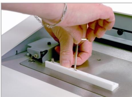
Secure the first rail; do not overtighten
