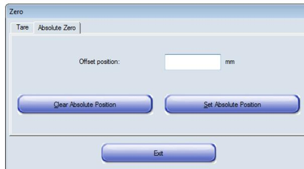
Using the onscreen keyboard, enter zero (0) and press the **Set Absolute Position** button, then **Exit**.
