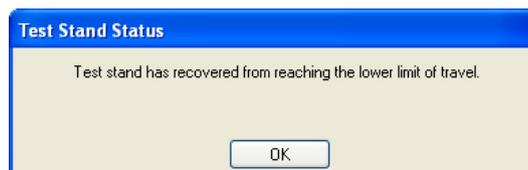
Press **OK** to acknowledge the warning and use the Jog buttons to move the crosshead so that you can then check the position of the limit stops and re-set if required.
