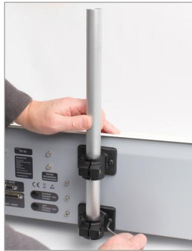
At this stage you can pass the USB end of the data cable up through the pillar, to save a trailing cable (see right, below).
