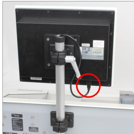
The console is powered from a separate adapter plugged into a mains socket.
