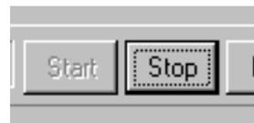
Clicking the **Stop** button in the workstation interrupts the measuring process immediately. The plate being measured is brought out to the loading position. You cannot resume measurement after clicking **Stop** but must begin the assay from the beginning if required.
