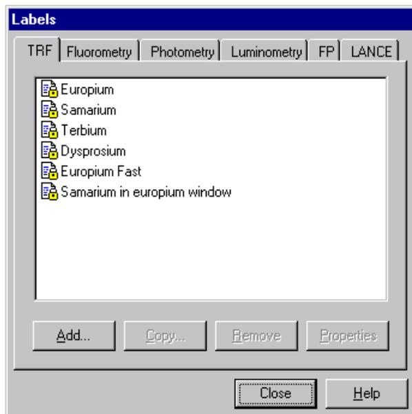
In this window there are tabs corresponding to the measurement technologies (labels) in the instrument. Each tab includes the names of the currently defined labels. Names of user defined labels can be freely defined by the user but names of factory pre-set labels cannot be changed. See the sections below for details.
