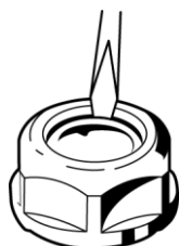
Figure 5-7 Stripping a seal ring
