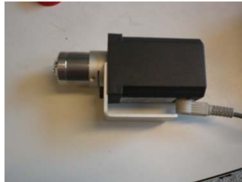
Fig. 2d, A 2 positions valve from VICI (EHMA)
