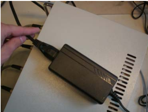
Fig. 2e, One of the 4 power supplies (GlobTek TR9Ci3200LCP-Y-2)
