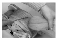
Turn the crank counter clockwise while lifting the batt from the drum. Use the doffer pin to keep the batt complete.
