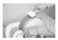
Clean the drum completely if you plan on using different colours or fibers next time.
