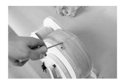
Filled up enough? Use the doffer pin to pull apart the carded fibers at the location of the wooden bar.
