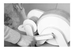
Let Hero pull the fibers out of your hand onto the small drum, while turning the crank clockwise.
