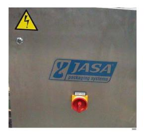
**8** Reset the machine: release the emergency stop button (**B**) then press "reset" and "OK" (see paragraph 4.1 on page 13).
