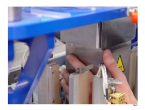
**14** Pick up the film with your right hand. Then pull carefully from left - right - left - right etc.
