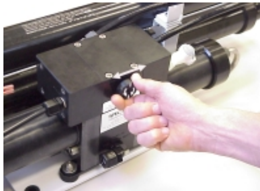
Open the pressure relief valve
