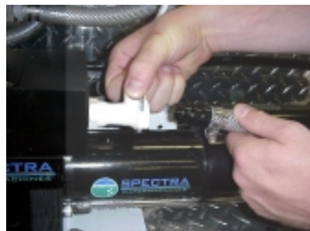
Connecting brine discharge hose
