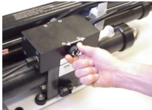
Open the pressure relief valve
