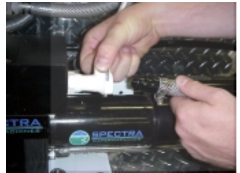
Connecting the Brine Discharge service hose.
