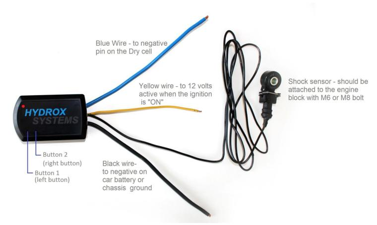
After you installed the HHO system in your vehicle, you have to connect the wires of the system. The Positive comes usually from the 12 or 24 volt + pin on the battery and goes straight to the positive pin on your Dry cell.
