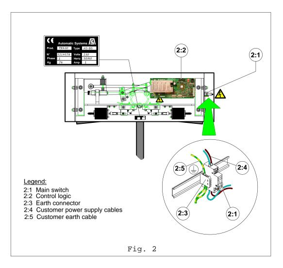
• As soon as you open the housing, put off the main switch (2:1) near the electrical control logic (2:2), located under the hood.
