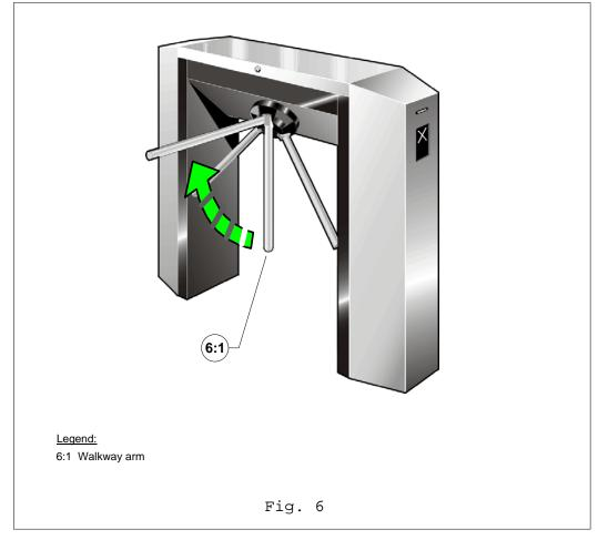
$\Rightarrow$  Lift up the walkway arm (6:1) manually and make sure this holds in the horizontal position.
