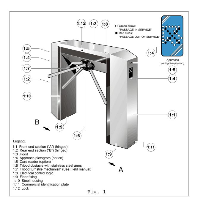
**Note**: Conventionally and as a general rule, the user will be considered in <u>direction "A"</u> when the turnstile is at his <u>right-hand side</u>, in <u>direction "B"</u> when the turnstile is at his <u>left-hand</u> <u>side</u>.
