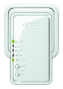
You can plug the LN-554 directly into a wall outlet. Switch the device on with the power switch located on the bottom of the device. The LN-554 automatically enters the self-test phase. During self-test phase, the Power LED will be lit continuously to indicate that this product is in normal operation.
