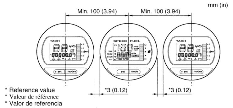
Install the meters 100 mm (3.94 in) or more from center to center of each meter. If installed closer than specification, the ring nuts can interfere with each other and prevent tightening.
