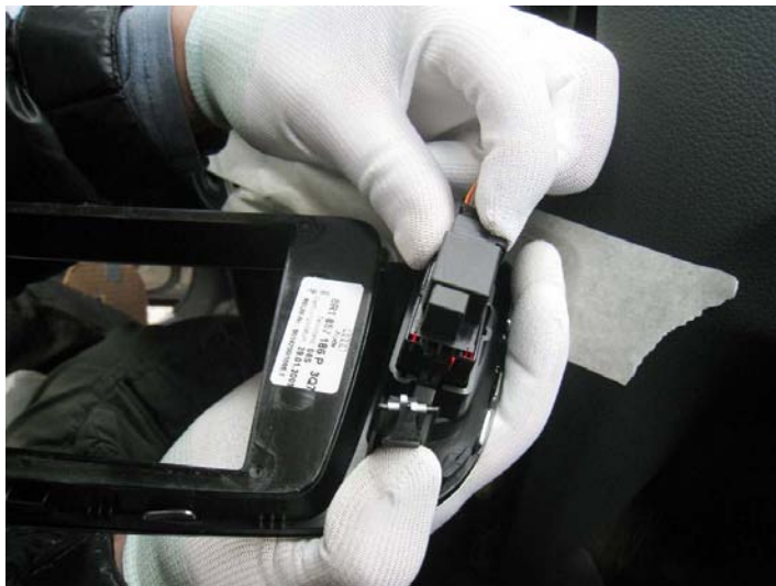
9. Disconnect wiring of monitor cover and emergency.
