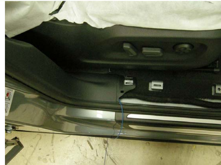
51. Wiring back signal wire.
