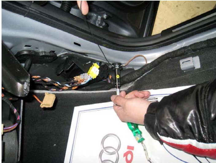
42. Main power ground point.
