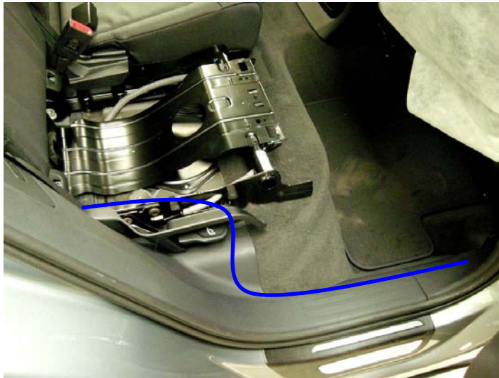
50. Wiring Back signal wire.
