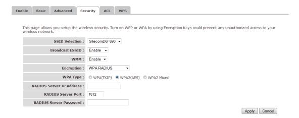
Wi-Fi Protected Access (WPA) is an advanced security standard. You can use an external RADIUS server to authenticate wireless stations and provide the session key to encrypt data during communication. It uses TKIP or CCMP (AES) to change the encryption key frequently. Press **Apply** when you are done.
