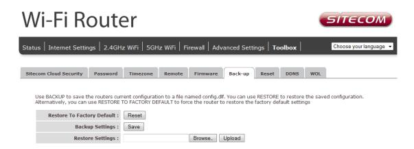
Use the "Backup" tool to save the current configuration to a file named "config.bin" on your PC. You can then use the "Restore" tool to restore the saved configuration to the router. Alternatively, you can use the "Restore to Factory Defaults" tool to force the router to perform a power reset and restore the original factory settings.
