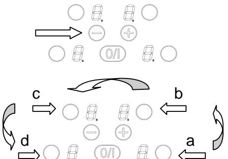
3) Remove your fingers from the touch control, press simultaneously [ + ] and [ - ]
