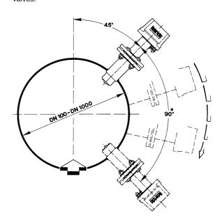
In order to stay within the indicated error limits, the installation must be performed according to EN 29104 "Measurement of Fluid Flow in Closed Conduits – Methods of Evaluating the Performance of Magnetic-Inductive Flowmeters." Based on this standard, the minimum straight run of pipe ahead of the inlet must be 10 pipe diameters (> 10 x DN) and 5 pipe diameters following the outlet (> 5 x DN) [DN = nominal diameter of pipe].
