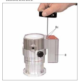
→ Remove the Electronic Drive Unit TC 100 (8) from the turbopump.
