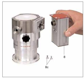
→ Assemble the new Electronic Drive Unit TC 100 (order number please see Section 10. Spare Parts) on the turbopump and connect again.
