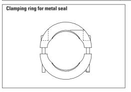
→ The screws on the clamping ring need to be tightened with a tightening torque of 3.7 Nm.
