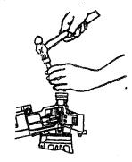
3. Remove jammed nail by using a rod bit it back to the nose.
