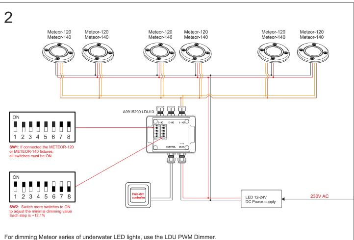
The 3 control outputs enable the dimming of 3 groups of underwater LED lights by using of one push-button switch.
