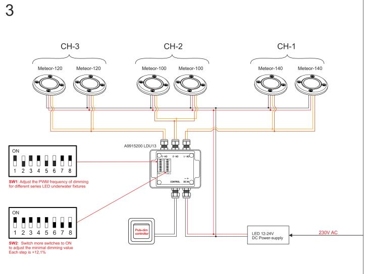
For dimming Meteor series of underwater LED lights, use the LDU PWM Dimmer. The 3 control outputs enable the dimming of 3 groups of underwater LED lights by using of one push-button switch. It is possible to control 3 different groups of underwater lights (for example: Meteor-100 & Meteor-120 & Meteor-140)
