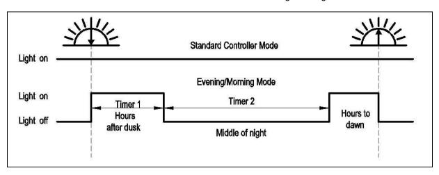
The ISC3040 recognizes days and night based on the solar array voltage. NLF will start when the PV(Voltage) < 10V.
