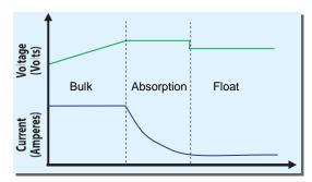
**Bulk:** This is the first stage where the battery is in a low charge state, (typically 10%), & receives the majority of its charge. During this stage the battery is brought to about 95% of its charge by getting 100% of the available solar power.
