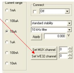
Channel selection can be automated in the Batchmode, similar to the HiMUX . The Loop command has a property "SetWE32ToIndex" that will set the channel nr to the loopcounter.
