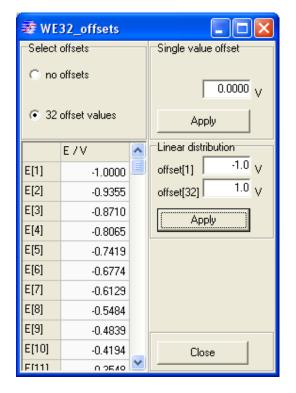
Note that when a MultiWE32 is used, there is no primary (base) electrode. For most applications, the offset potentials would remain at 0V, because potential manipulations are more conveniently done by setting the base potential.
