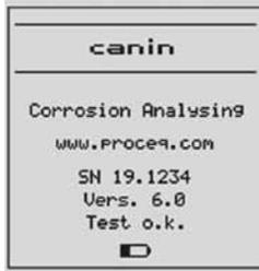
It will start up in whichever mode was used last. For potential measurements the instrument must be in “Corrosion analysing” mode.
