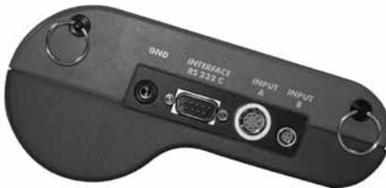
Rod electrode connects to INPUT A and also requires GND connection.
