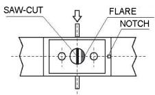
Set both the valve as well as the actuator in OPEN position by hand and after electrical actuator construction, back in approx. 45° position.
