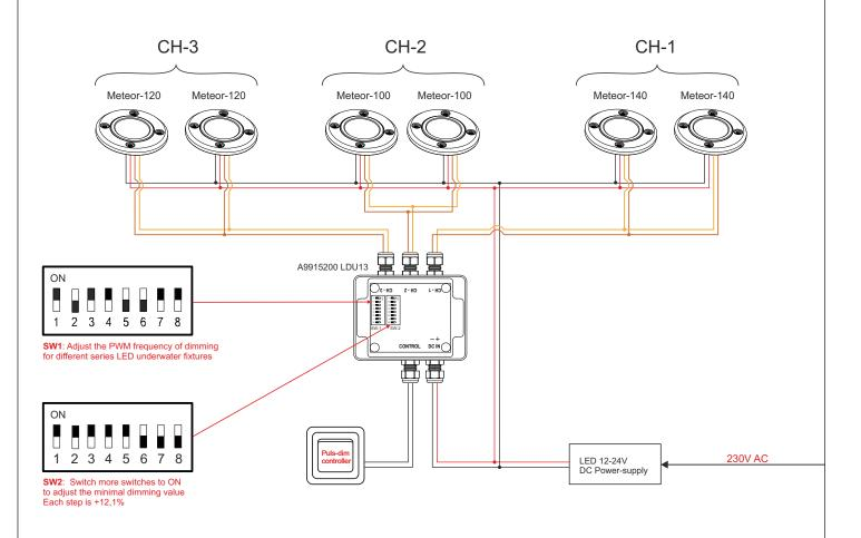
For dimming Meteor series of underwater LED lights, use the LDU PWM Dimmer.
