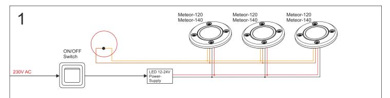
**Note:** If the remote control is not used for dimming operation the both CONTROL wires have to be bridged and insulated or connected to the GND.
