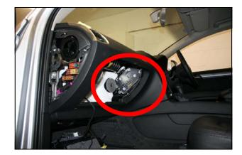
The screen control unit on new A4 and A5 is located behind the CD changer and heater controls. The CD changer is removed with AUDI removal keys.
