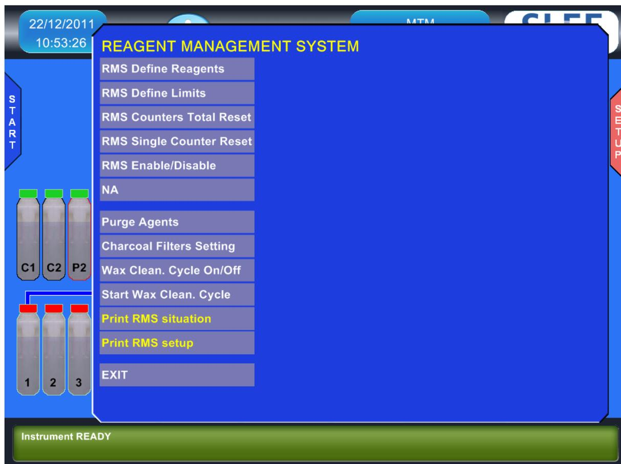
The MTM II RMS is a system to punctually and exactly manage all reagents to guarantee a constant process and sample quality. The use of the Reagent Management System eliminates the need to make annoying written annotations of reagent bottle status. This results in substantial time savings and eliminates the possibility of errors caused by multiple operators using the instrument.
