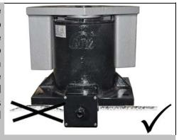
It is mandatory to use fastening screws of the quality 8.8 (DIN 931 or 933) and secure them with counter nuts (DIN 934) and a suitable glue. The screws have to be checked and possibly retightened at regular intervals (generally once a month).
