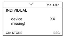
When the ballast address of the missing device is determined, press **OK** to transfer its backup data to memory for further processing.
