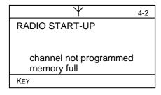
If all 200 channels that could be stored in a central controller are occupied the depicted error message is displayed.
