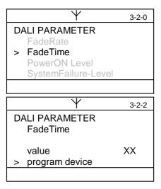
The fading time is given by the "FadeTime" value.
