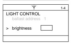
Following the cursor changes to the menu point *brightness* automatically. Now the brightness level (0 - 100 %) can be entered and confirmed with **OK**.
