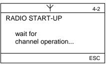
The central controller now waits for a radio telegram from a radio transmitter. This is sent by pressing the button that should be learned for a longer time or by inserting the batteries in a sensor. (For further details please have a look at the instruction manuals of the corresponding transmitters)
