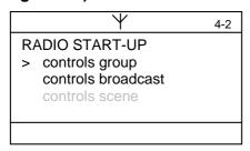
Dependent of the transmitter type or of the radio telegram type a menu choice is displayed. Here a selection is made whether group-, broadcast- or scene-control is linked with the corresponding radio telegram. The according menu point is selected with the cursors and confirmed with OK. At controls group and controls scene the desired group or scene number has to be entered and confirmed with OK on the next screen
