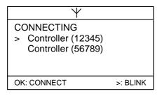
Subsequently the display shows a list of central controllers found. With the buttons • a central can be selected. To check whether the correct central is selected, blinking of all fixtures connected to the selected central can be initiated with the • button. If the desired central is found, confirm selection with OK.
