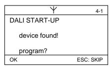
When the device is found the lamp connected to it flashes. Press OK to start the programming of this device. Should the fixtures be programmed in a special order (e.g. corresponding to the mounting place), the actual blinking device can be skipped with the ESC –button and programmed later on.
