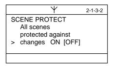
Coming from the Main Menu call up submenu service .. / DALI system .. / scene .. / Scene protect. The actual setting will be displayed. Select entry with OK, enable (ON) /disable (OFF) scene protect with the buttons ▲ and ▼ or 1 and 0.
