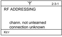
If a channel is to be unprogrammed that has not been programmed in the central controller, the depicted message will be displayed.
