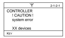
If the transmission routine detects an error in the DALI SYSTEM, a new startup process must be carried out.
