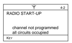
If eight light sensors or presence detectors have already been programmed and an attempt is made to train a further light sensor or presence detector, this error message is displayed.
