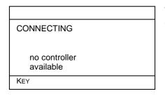
The HPT could not establish a radio link to a central controller.
