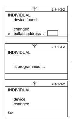
After successfully searching, the system suggests the ballast address of the previously demounted faulty as the replacement. \_\_\_
