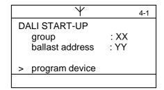
The group number entered XX and an automatically generated ballast address YY are displayed. Desired group number and ballast address can by selected and edited with the cursor control. Programming is started with the OK button (it is urgently recommended to note the group resp. ballast address of every device for documentation of the installation.)
