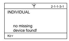
A missing device could not be found when searching for a missing device in the exchange device menu option.
