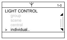
With the menu point *individual* in the LIGHT CONTROL menu individual fixtures can be controlled. For this select the corresponding entry with the cursor buttons • and press **OK**.
