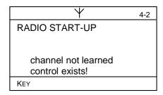
If a light sensor or presence detector is to be assigned to a group that is already being regulated by another light sensor or presence detector, the depicted message will appear.
