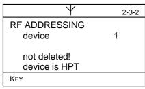
If an attempt is made to delete the HPT currently connected to the central controller, the message alongside will appear. You cannot delete an HPT.
