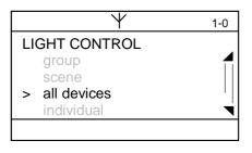
With menu point *all devices* in the lighting control menu, the whole installation can be controlled. Please select the corresponding line with the cursors ▲ ▼ and confirm selection with OK.
