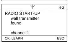
After successful reception of radio telegrams the transmitter type (here: *Wall transmitter*) and the functional type (here: *channel 1*) is displayed. Press **OK** to learn this transmitter or reject it and wait for next transmitter with a short press on **ESC**.
