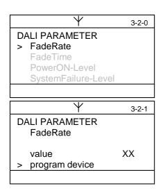
The dimming speed for manual operation dimming is given by the *,FadeRate'* value.
