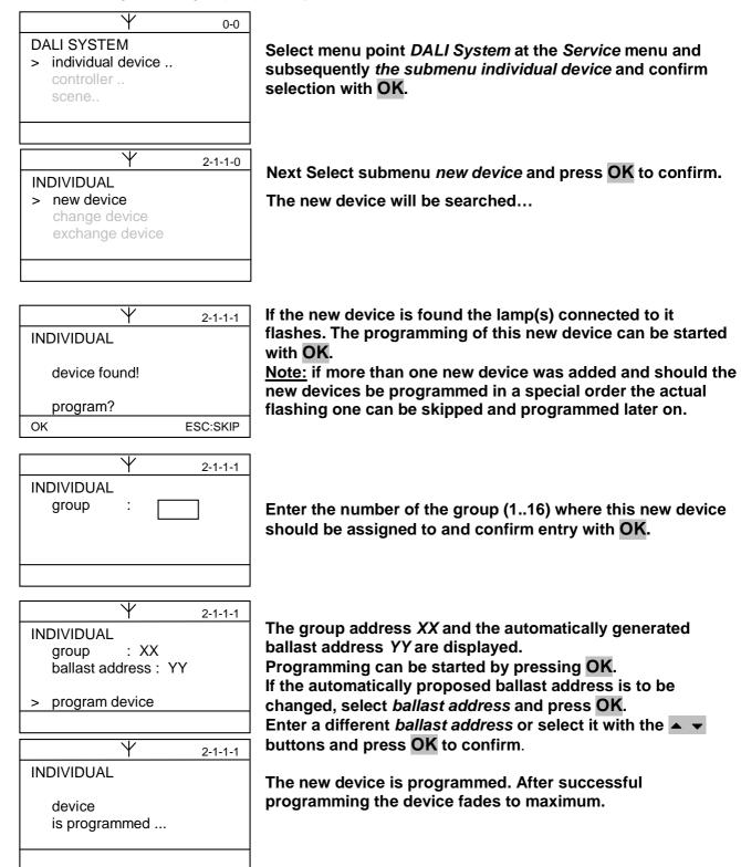
If no new device is found please check if it is correctly connected to the controller and the line voltage and if it reacts to the central On/Off/Dimming functions of the HPT. Is the connection correct, but the device is still not found, it was obviously programmed before. In this case please follow the instructions on next page.
