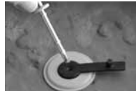
Remove rod after concrete hardens
