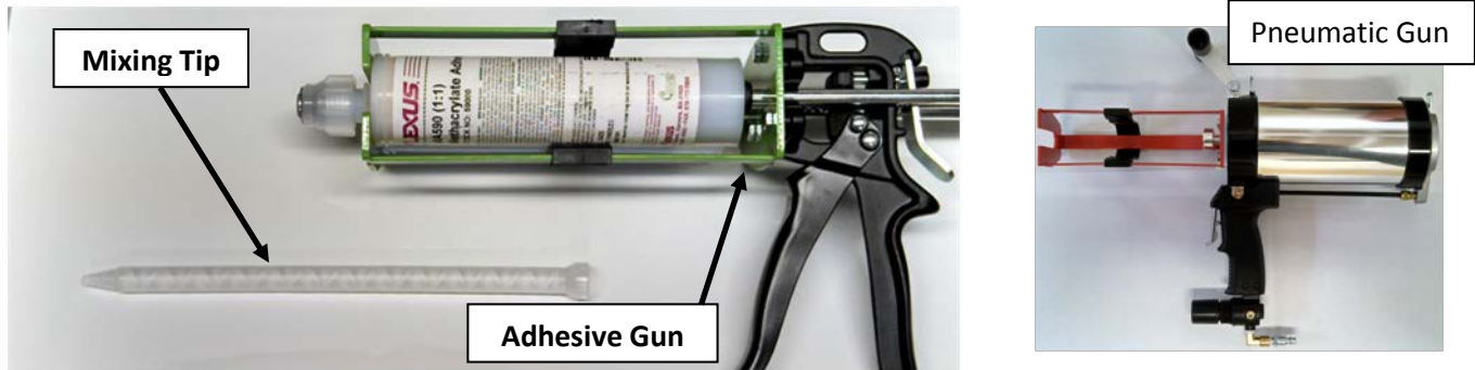
FIGURE 12 – ADHESIVE INSTALLATION SUPPLIES
