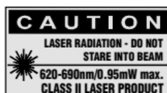
laser class II according CFR 21, § 1040 (FDA)
