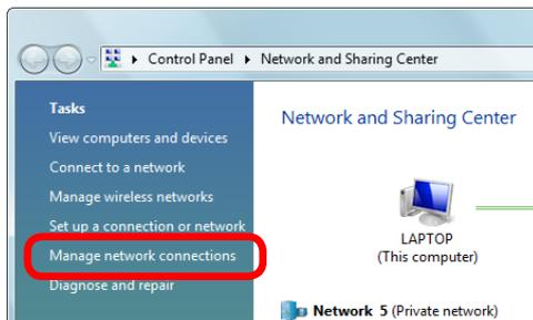
Windows Vista: Go to *Start>Control Panel>Network and Internet>Network and Sharing Center>Manage Network Connections*.
