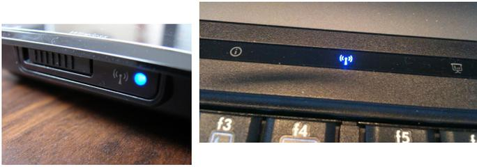
Example of a slider and a touch button with activated light.
