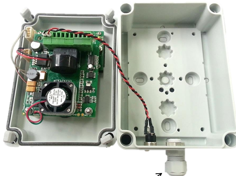
Cable gland for RS232 or RS485 connection
