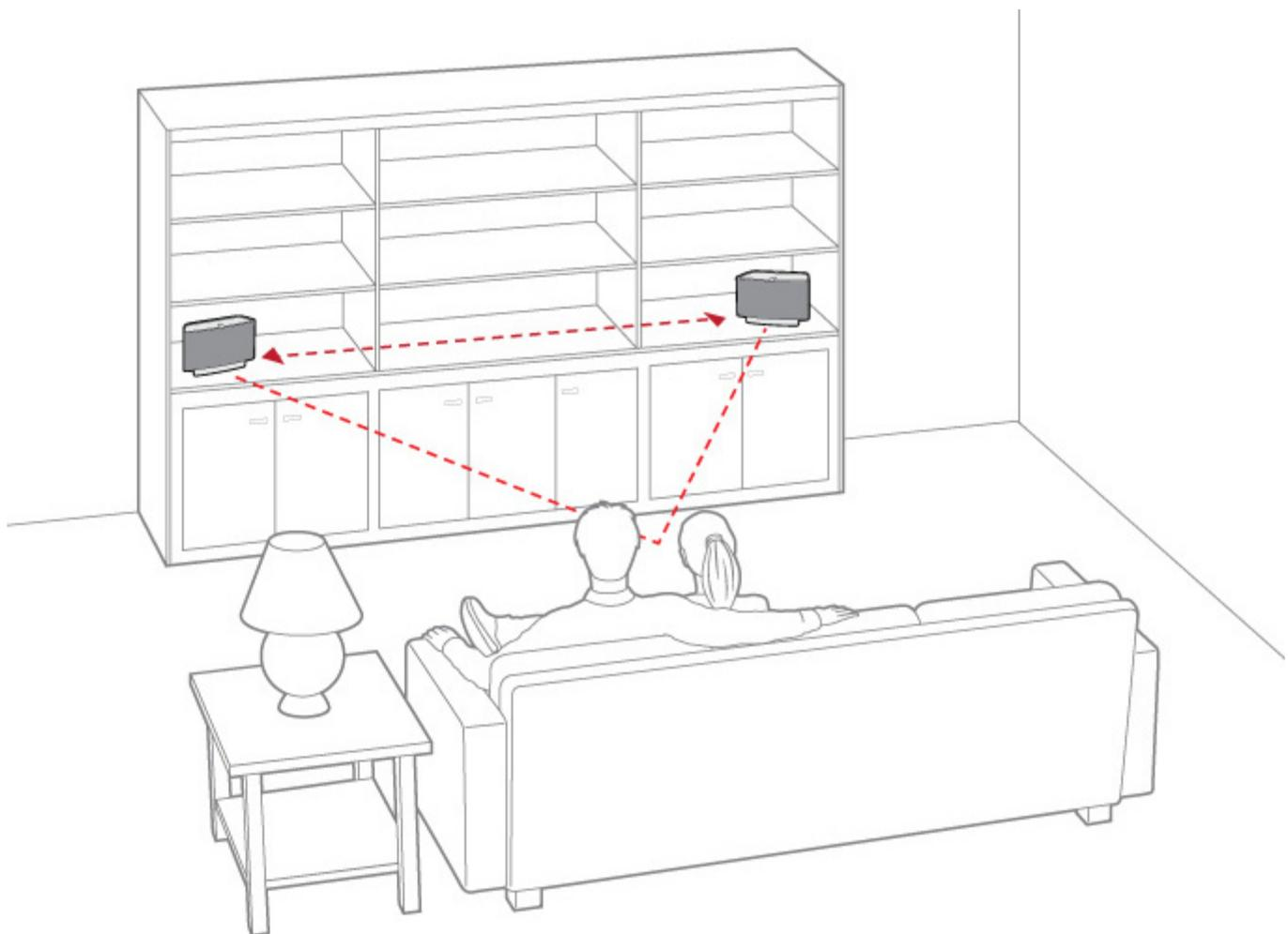
**Note:** The Stereo Pair setting is for use with PLAY:3 and PLAY:5 units only. Both Sonos components in the stereo pair must be the same.
