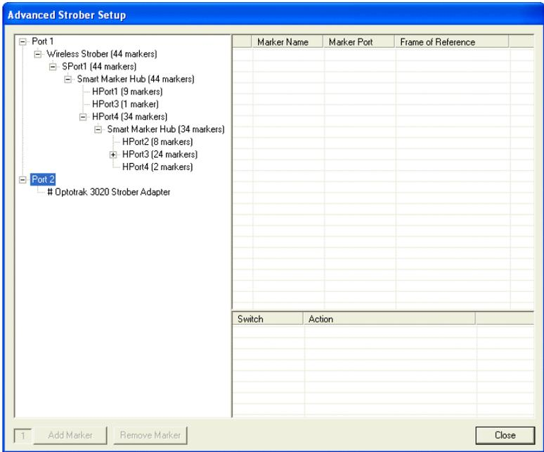
Figure 7-5 Wireless Strober Setup
