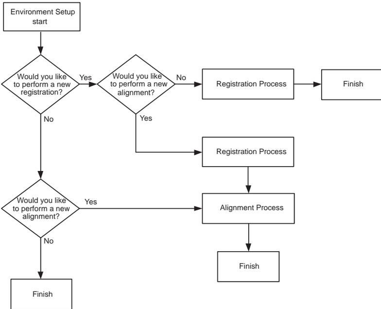
Figure 3-1 Environment Setup Process
