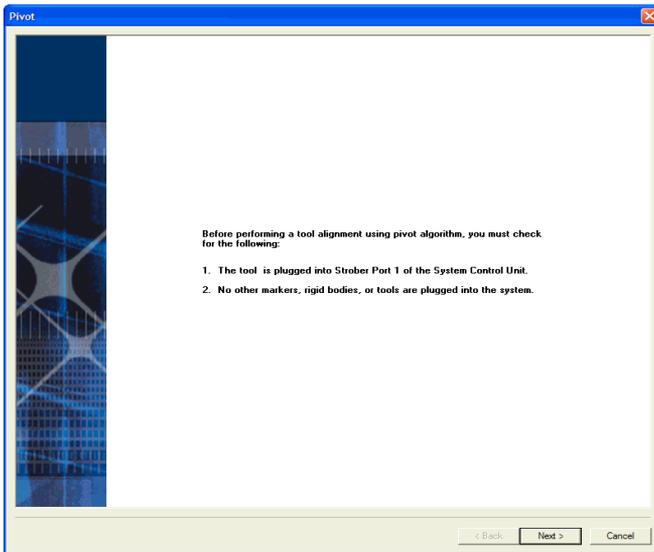
Figure 9-1 Pivot Procedure - Initial Dialog
