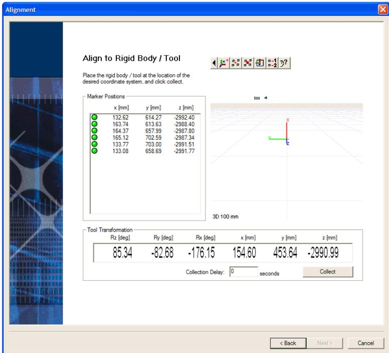
Figure 5-7 Alignment — Collect Alignment Object Data
