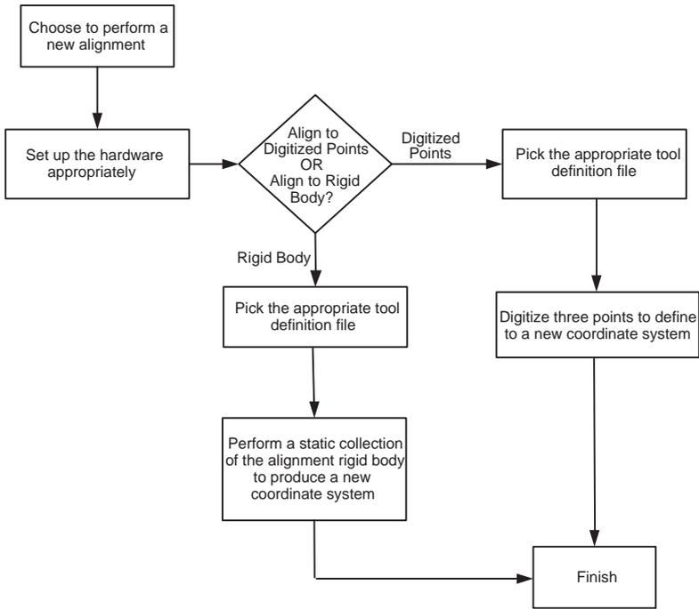
Figure 5-1 First Principles Alignment Procedure
