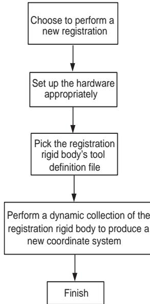
Figure 4-1 First Principles Registration Procedure
