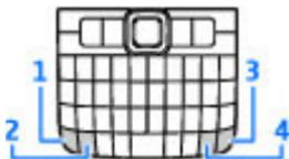
1 — Function key. To enter digits or characters printed on the grey part of the keys, press and hold the function key and press the corresponding key, or press and hold the corresponding key only.
