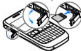
2. Insert the memory card in the slot with the contact area first. Ensure the contact area is facing the connectors on the device.
