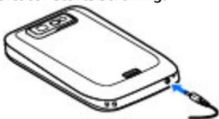
3. When the battery is fully charged, disconnect the charger from the device, then from the wall outlet.
