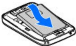
5. Close the back cover, and lock the back cover release button.
