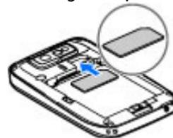
4. Insert the battery. Align the contacts of the battery with the corresponding connectors on the battery compartment and insert in the direction of the arrow.
