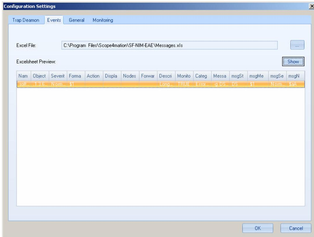
Selecting Configuration > Events opens the dialog above. If you need to use a predefined event configuration then here is where you need to point to the correct file. Click “Show” to see if the file is usable by the NIM EAE. This is also the file that is used to save changes to the event configuration. So when starting out just leave this settings page default. The file is automatically created if not present when event configurations are made.
