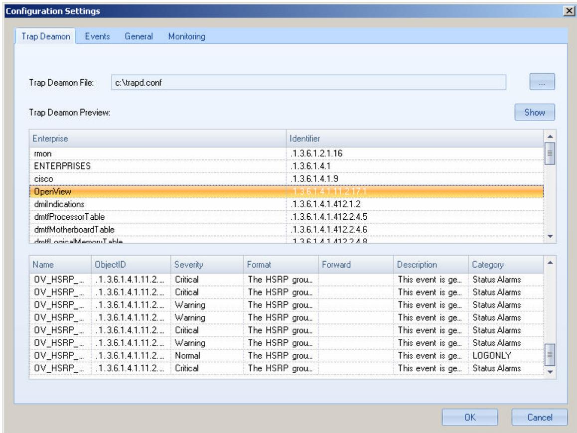
Selecting Configuration > Trap Daemon opens the dialog above. Browse (with the “...” button) or manually enter a path to a valid trapd.conf. Then click “Show” to display the contents. If the contents are shown then Trap Daemon configuration page is set correctly provided the trapd file is correspondent with the trapd.conf in the related NNM environment.
