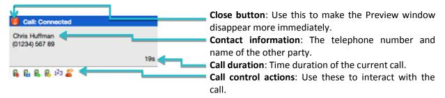
As you can see Preview window allows you to interact with the current call in a number of ways. One of the most common ways is to click on the new contact or Edit contact button to apply a name to the person you are speaking to. This is covered in a later section, <u>Address books</u>.
