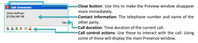
The actions at the bottom of the Preview window adapt to the state of the call. The example picture shows the actions that are available when a connected call is in progress.
