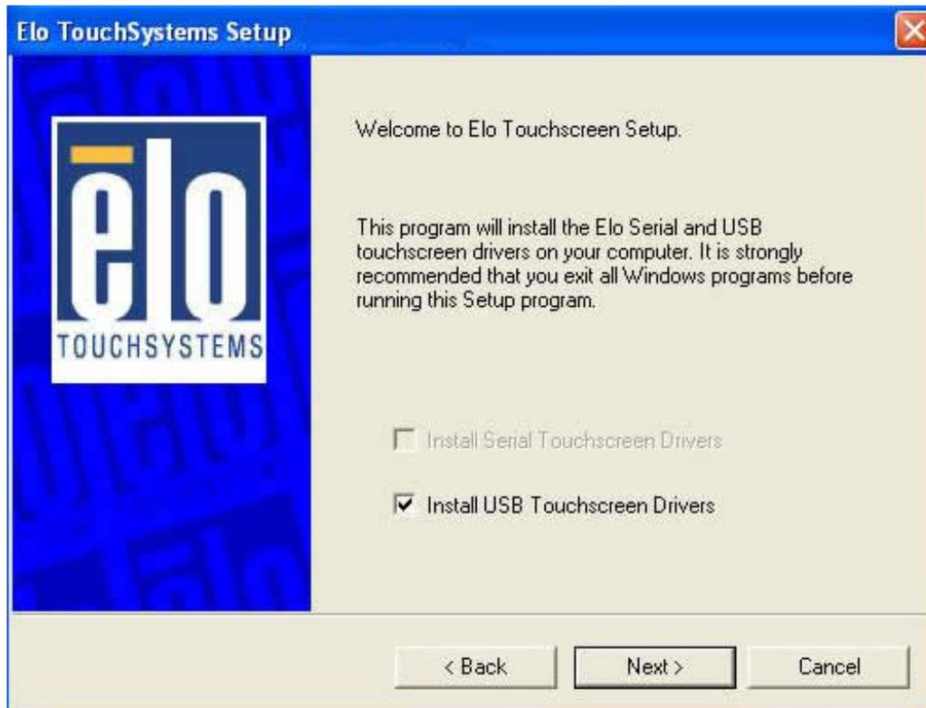
When a new APR monitor is first installed on a PC, you may see the following dialog box while the driver is reading the information from the sensor. This process may take up to 4 minutes before touch begins to work.
