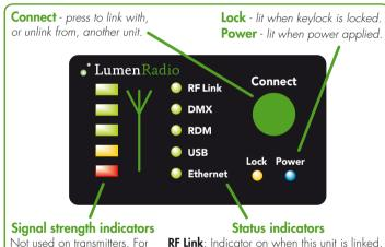
Not used on transmitters. For receivers, the amber indicator turns on at roughly 20% of maximum signal strength and the top green indicator turns on at roughly 90%. The red indicator turns on only if a problem occurs with the link to the transmitter.
