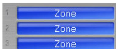
Zone button: Push to select a room /zone (button turns into green). Push and hold until the button changes to red, to block a room/zone for paging/messaging
