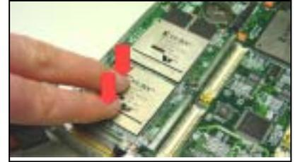
8. Using a flat-bladed screwdriver, begin to tighten the DIME-II Fixing Screws. Tighten the screws alternately, tightening each screw one turn, before swapping and tightening the opposite screw by one turn, until both are fully tightened.
