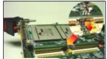
7. Apply light downward pressure to the module. While still holding it in place, proceed to step 8.
