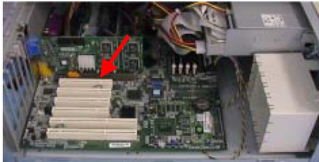
3. Fit the BenONE - PCI into the PCI slot you have selected and push down firmly:
