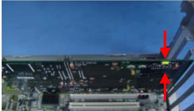
The hardware installation of the BenONE - PCI is now complete. It should be noted that at this stage the card will not function, until the BenONE - PCI drivers and software have been installed. Instructions on how to do this are given in 'Software Installation' on page 25.
