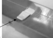
Rear-panel attachment clips are now engaged ("B"). If needed remove any paint drippings from below the clips.
